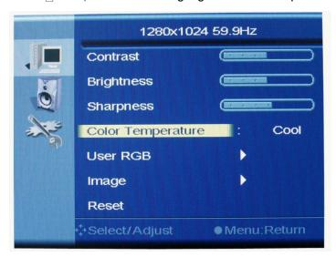
b. Press "1" to select preset color temperature settings, like Cool, Natural, Warm, or select User to adjust Red, Green, Blue independently. If Cool, Natural, or Warm is selected, then press "2" to confirm the selection and press "2" to exit.
